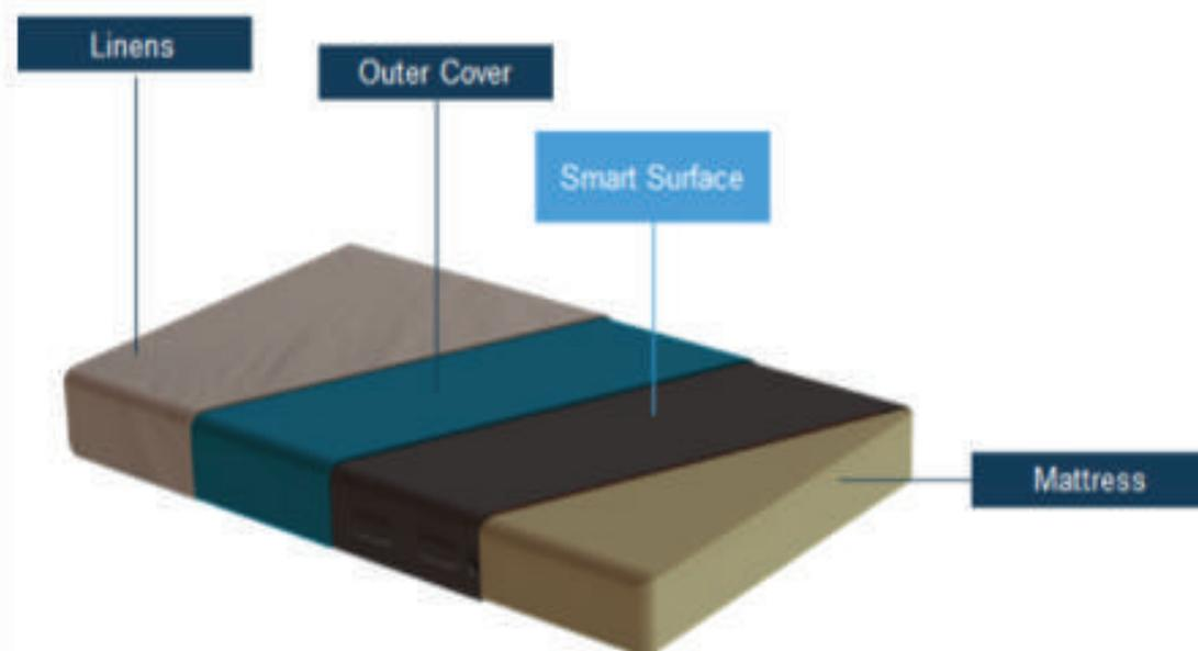
**Figure 1** A cross-sectional view of PI-Connect installed over a mattress. PI-Connect comprises an array of sensors embedded in a thin, flexible surface placed underneath the bedsheet. It is not in direct contact with the patient
